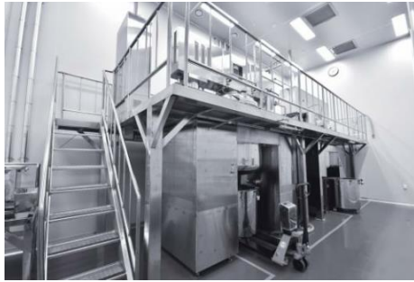
Melting tank(1,000L / 500L)
