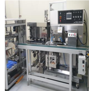
10 row stick packing machine(810,000 bags/ 8H)
