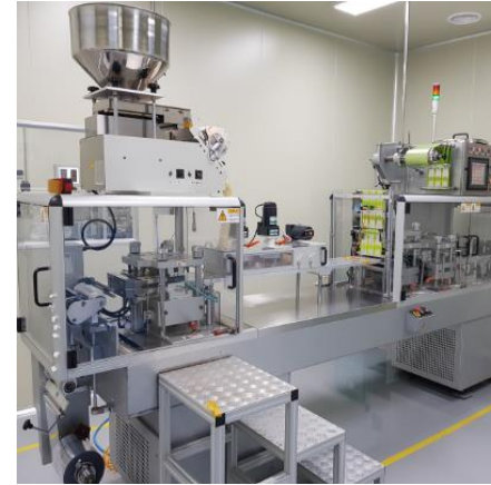
PTP packaging machine (60,000 packs/8H)
